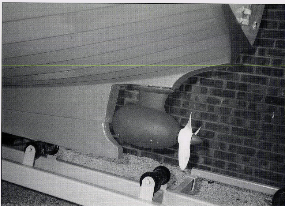
Dynia's Accumot pod-motor mounted underwater.
