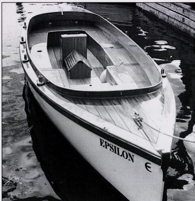
Note the control pedestal and louvred motor housing
