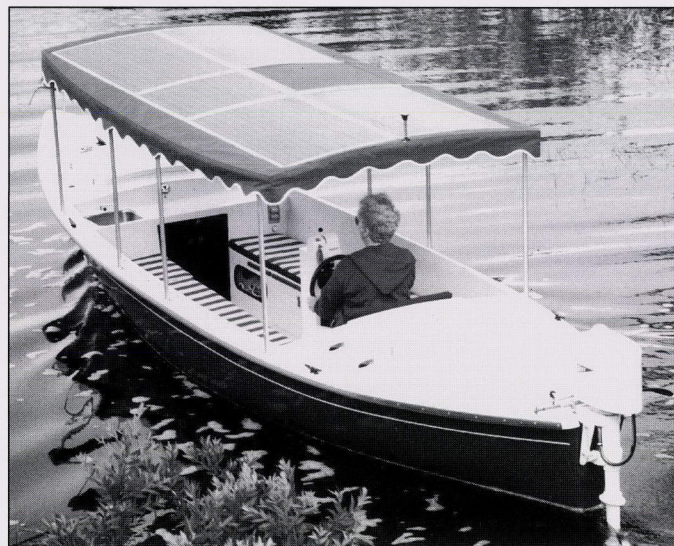
The Ray Explorer with four 90 watt solar panels and a smaller auxiliary battery panel
