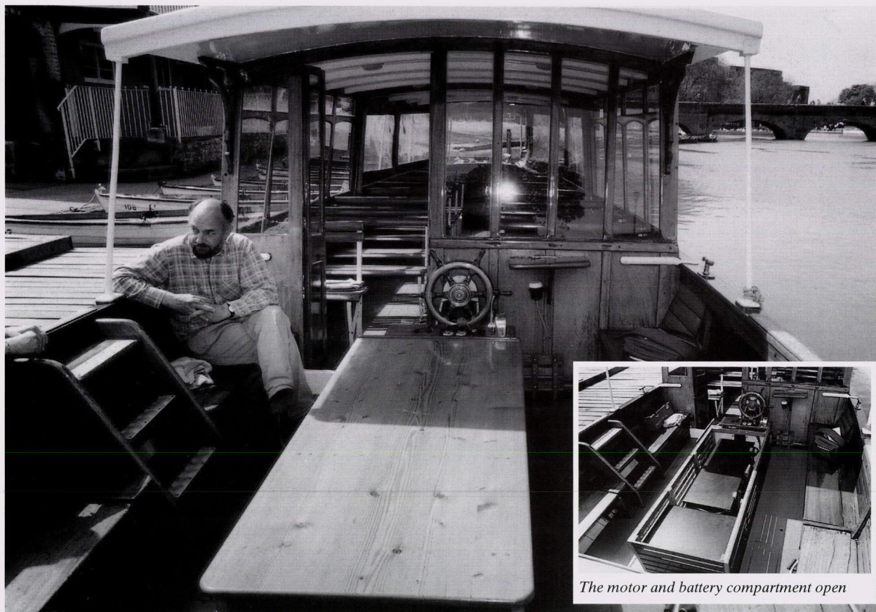
Proprietor Edward Rose beside the motor and battery compartment doubling up as a vibration free table/seat in the centre of the boat
