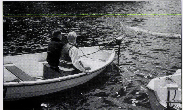
The bow mounted electric outboard from the Lakeland Electric Boat Centre.
