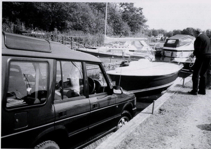
The front tow hitch provides a high degree of control when launching
