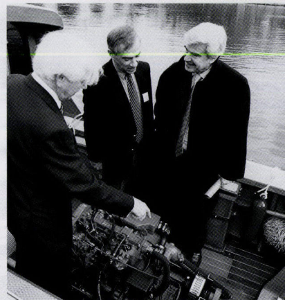
On board the Environment Agency's patrol launch Colne, the Minister is shown the diesel / electric system, and its tiny electric motor that replaces the diesel engine for normal cruising
