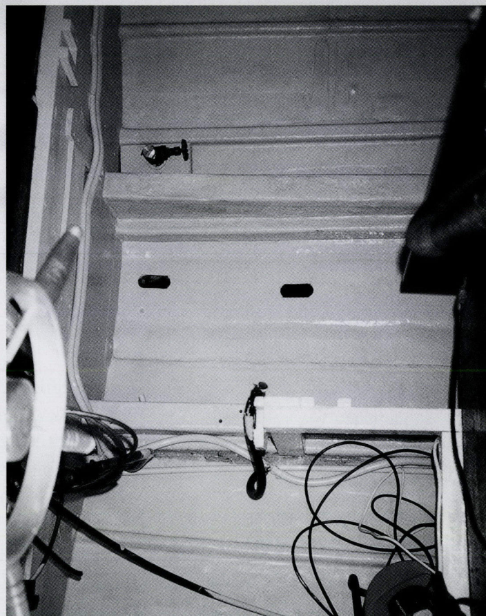
The space left after removing the diesel engine
