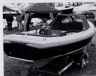
The Interboat 19, available in either electric or diesel from the Thames Electric Launch Company
