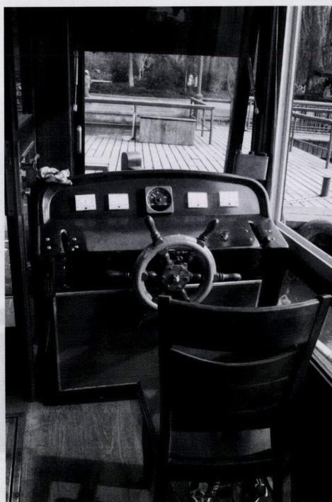
Helmsman's station 100A ammeter and 120V voltmeter for each motor flanking rudder angle indicator
