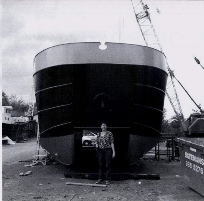
Bow view of Solaris, showing the catamaran configuration of the hulls
