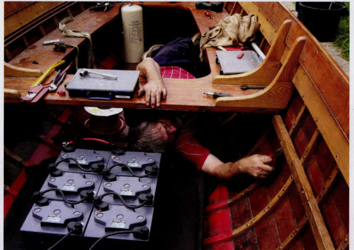
Removing old steam clips (batteries in temporary installation on old boiler tray)
