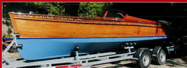
MAGNA CARTA: 25ft Slipper Launch by P. Freebody & Co. 1992. Nexus 2kw motor.
